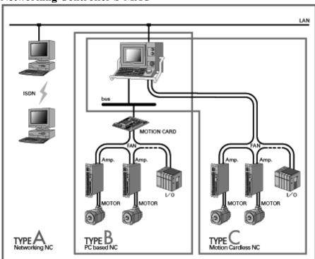
We released S-MAC networking controller in June 1997, that uses SERCOS and CAN (DeviceNet, etc.) as the field bus and has open-architecture support. The basic specifications of TYPE A, TYPE B and TYPE C have been settled.
